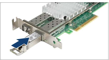
Figure 47: Inserting the SFP+ transreiver
